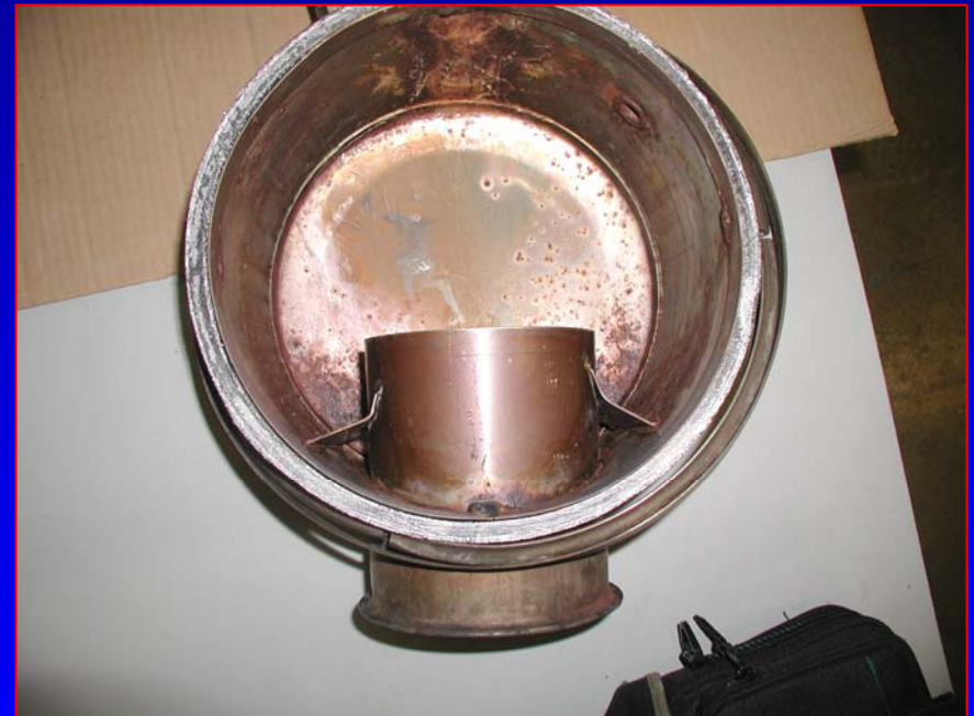
Filter Outlet Section
