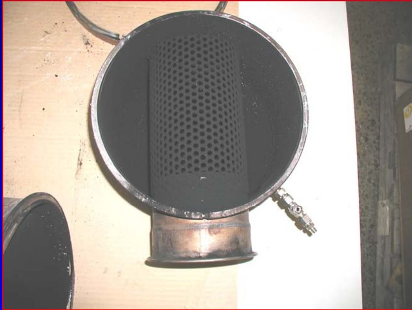
Filter Inlet Section
