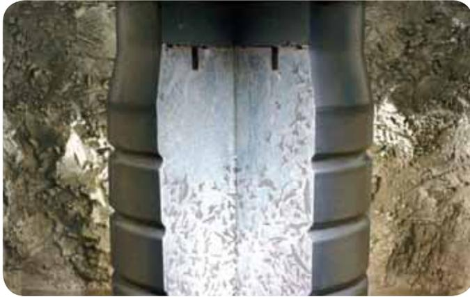
Cut through a barrel containing intermediate level liquid waste solidified in concrete. Intermediate level waste consists of heavily contaminated materials, such as fuel rod casings or decommissioned parts of the reactor vessel. This waste requires radiation shielding. Storage time will depend upon which radioactive isotopes are present in the waste. Radioactive liquids are solidified before disposal. *Credit: Dounreay*
